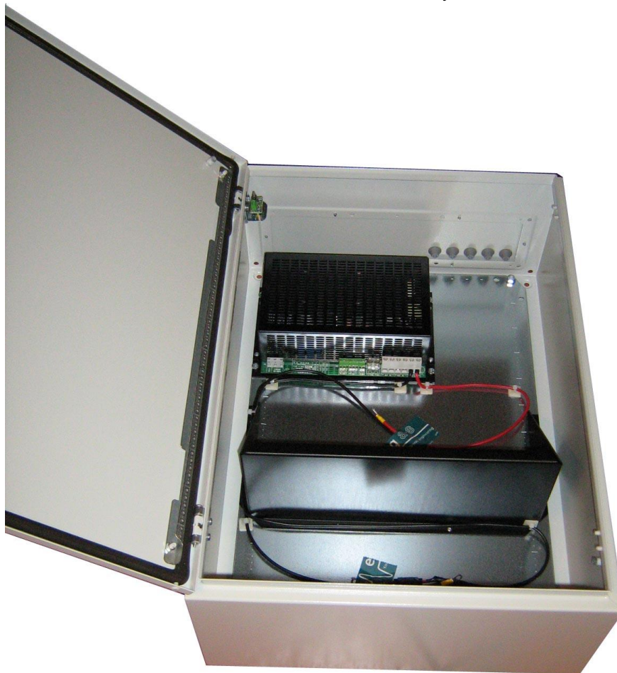
Picture show wall mounted enclosure without batteries. Battery bracket is fitted for 2 x batteries of 12V 70Ah.
